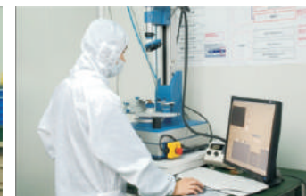
偏心检测 Eccentricity Inspection
